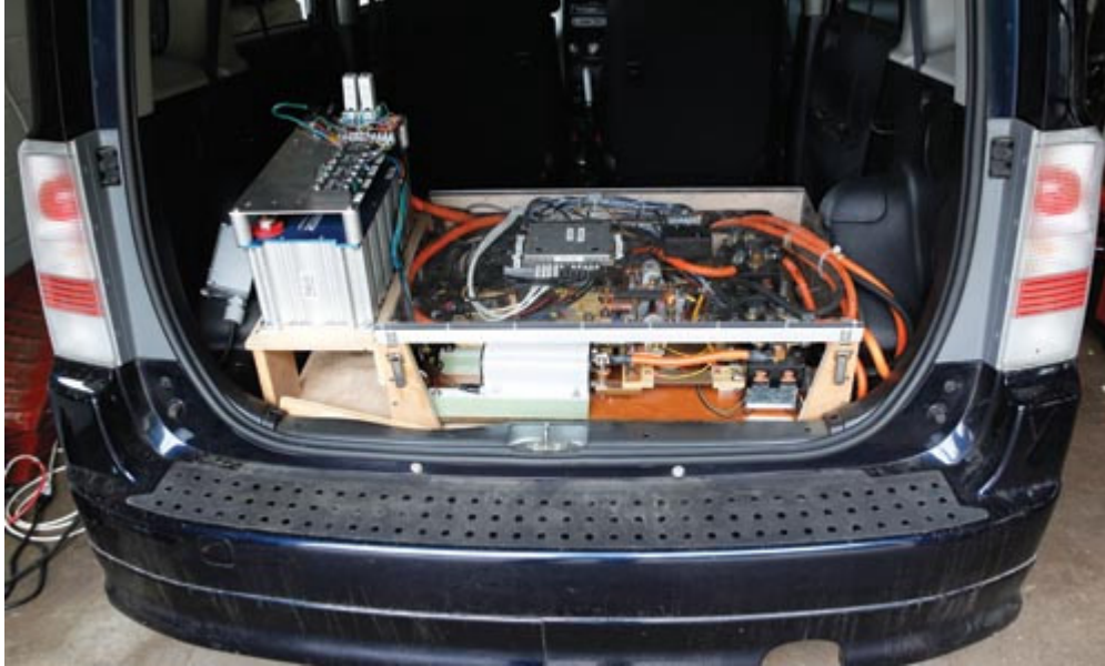
Under the Scion's rear hatch; the raised assembly at left includes the supercapacitor. Heather Mull
